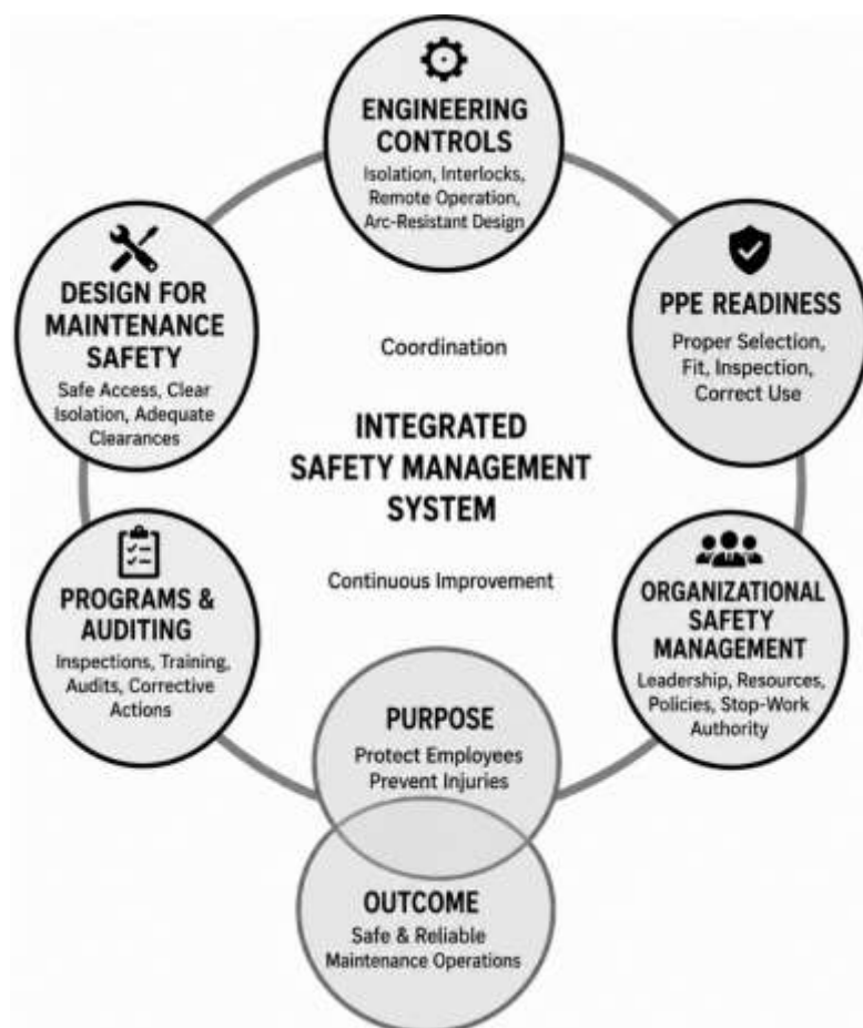
Figure 5: Integrated Engineering Controls, PPE Readiness, and Organizational Safety Management Framework for Industrial Maintenance
