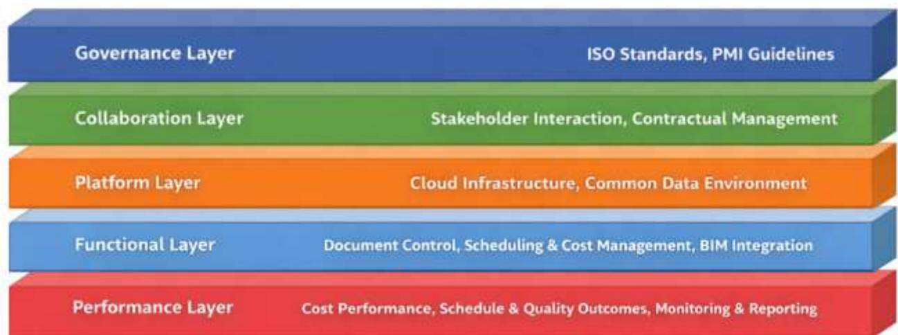
Figure 1: Architecture/Layered Model of DCMF Components
